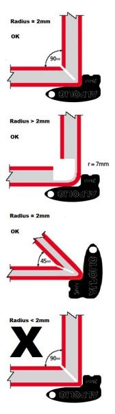
A bend radius of less than 2mm may cause the finish to crack and will void the finish warranty.
